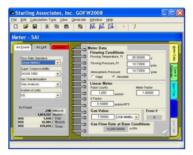
The volume at flowing conditions is converted to base conditions using the supercompressibility method specified.
