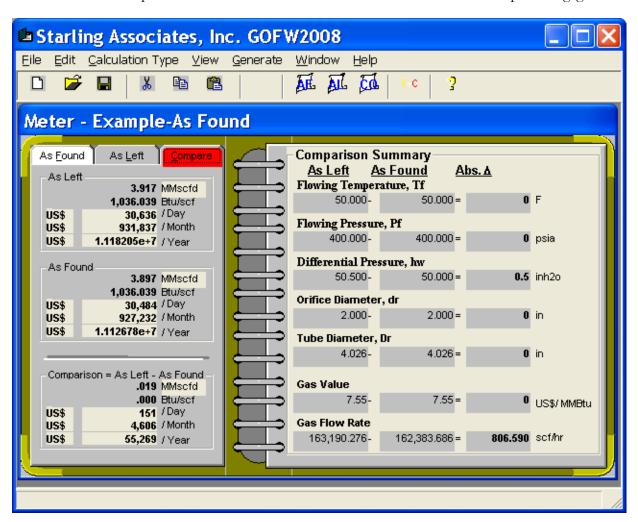
Notice on the Compare screen that the increase in Differential Pressure  $h_w$  from 50.0 to 50.5 inches of water yields an increase in the calculated Gas Flow Rate from 3.897 to 3.917 MMscfd. The Gas Analysis used (viewed by clicking the Gas Char tab) yields a calculated Gross HV = 1036.04 Btu/scf (viewed by clicking the meter Data tab then clicking the "dog ear" on that page to reveal the second
