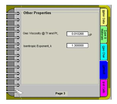
Section 3.4.5 of AGA Report No. 3 (1992) notes that the default value for viscosity is an average value for natural gases with relative density from 0.55 to 0.75 in the temperature range from 30 to 90°F. For gases with viscosity outside the range 5.9E-6 to 7.9E-6 pounds mass per foot-second and/or flow outside the above ranges, particularly at low Reynolds numbers, the default value should be replaced by a more accurate gas viscosity input value.
