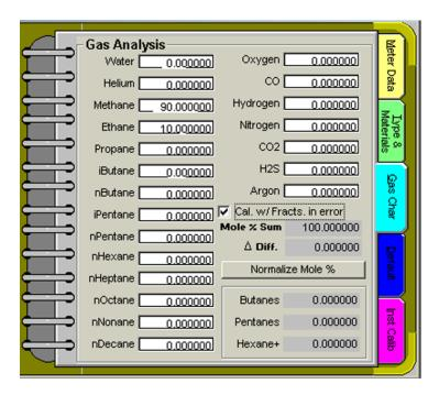
The Gas Analysis screen permits the user to enter values for 21 components. However, when the Gas Analysis Method under AGA8 1985 or NX19 1962 is used argon is excluded.
