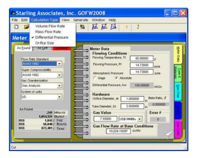
➤ **GOFW2008** will only perform Differential Pressure calculations in US units. Additionally "User Input" Super Compressibility may not be used for Differential Pressure calculations.
