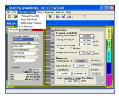
➤ **GOFW2008** will only perform Orifice Size calculations in US units. Additionally "User Input" Super Compressibility may not be used for Orifice Size calculations.
